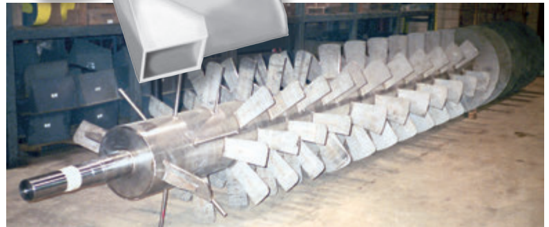
30' long, 48" diameter 316SS paddle type screw
