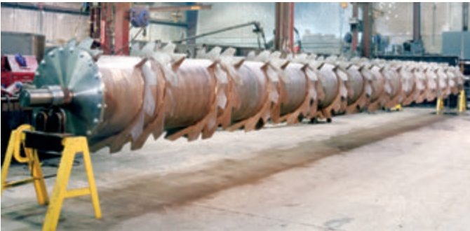
36' long, 38" diameter 2205 duplex SS pulp screw
