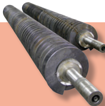
30' long, 48" diameter 316SS paddle type screw
