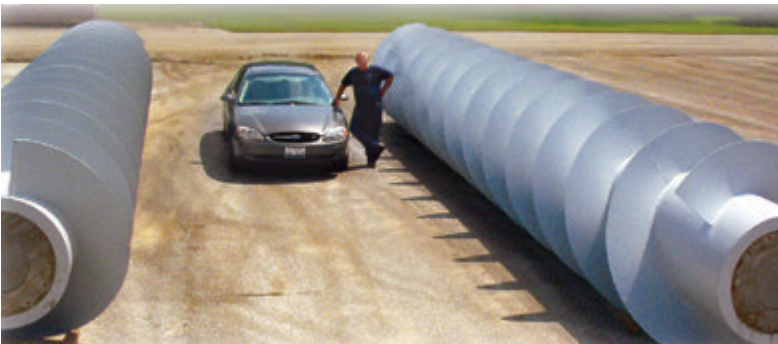
46' long, 78" diameter double lead water lift screws
